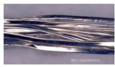
especially at contact points. MADEIRA's highly conductive embroidery thread does not only offer specific technical functionality but also retains its textile characteristics such as flexibility, resilience and easy processing.
