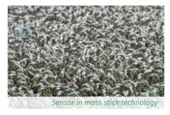
**HC40** and **HC12** are skin friendly, comfortable, biocompatible, washable and therefore ideal for Smart Textile applications. Amongst all metals, silver offers the highest electrical and thermal conductivity. In addition, it has antibacterial and antistatic properties.
